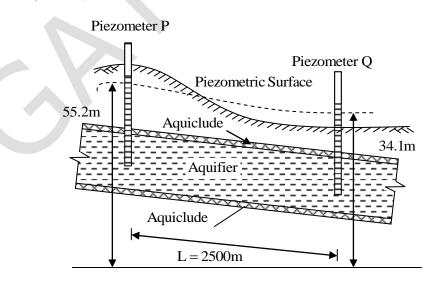
The heads indicated by two piezometers P and Q are 55.2 m and 34.1 m, respectively. The aquifer has a hydraulic conductivity of 80 m/day and its effective porosity is 0.25. If the
