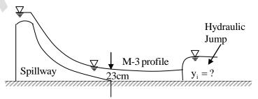
The flow enters as an M-3 profile in the long wide rectangular channel with bed slope  $\frac{1}{1800}$  and Manning's n = 0.015. A hydraulic jump is formed at a certain distance from the foot of the
