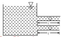
For parallel connection total head loss due to friction
