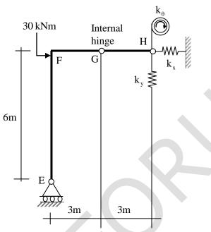
For the externally applied moment of 30 kNm at node F, the rotation (in degrees, round off to 3 decimals) observed in the rotational spring at node H is \_\_\_\_\_.
