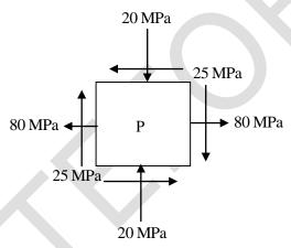
By how much angle ( $\theta$ ) in degrees the stress element should be rotated in order to get the planes of maximum shear stress?
